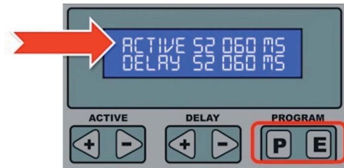
FIGURE 2: Selection of the current duration of each column (60ms), and of the relaxation time between the columns (60ms).
